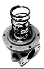
**15.** Refit the upper wastegate cap re-using the 6mm Allen head screws. Use Loctite or a similar thread locking product on these screws.
