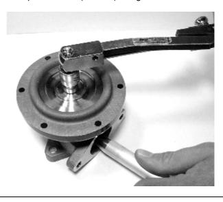
**13.** Align the six holes on the outer ring of the wastegate diaphragm with the 6 holes in the lower wastegate cap.
