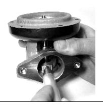
**6.** Remove the M6 GlennLock nut using a 10mm wrench or spanner and discard.
