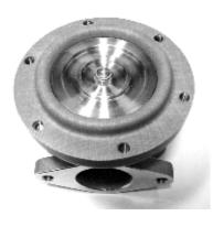
**14.** Select and fit the required wastegate spring or springs to the upper diaphragm spring support. See (spring info) for information on wastegate spring identification.
