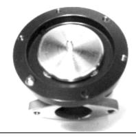
**10.** Refit the wastegate diaphragm, smooth side down, with the moulded roll facing upwards as shown below.
