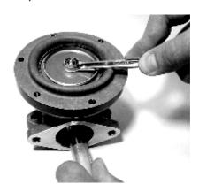
**7.** Remove the pressed upper diaphragm spring supports and discard.
