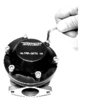
**3.** Remove the wastegate spring and inspect the upper diaphragm spring support.
