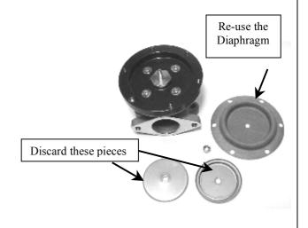
**9.** Fit the new billet machined lower diaphragm support with the smooth side up and the lipped side facing down.
