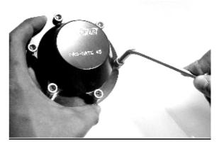
**3.** Remove the wastegate spring and inspect the upper diaphragm spring support.
