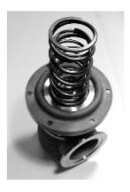
**15.** Refit the upper wastegate cap re-using the 6mm Allen head screws. Use Loctite or a similar thread locking product on these screws.
