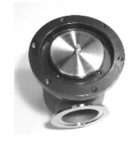
**10.** Refit the wastegate diaphragm, smooth side down, with the moulded roll facing upwards as shown below.
