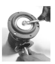
**7.** Remove the pressed upper diaphragm spring supports and discard. Carefully remove the wastegate diaphragm.
