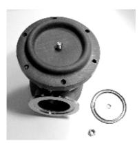
**8.** Remove the pressed lower diaphragm spring support and discard.
