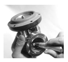
**6.** Remove the M6 GlennLock nut using a 10mm wrench or spanner and discard.
