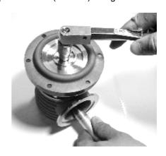
**13.** Align the six holes on the outer ring of the wastegate diaphragm with the 6 holes in the lower wastegate cap.
