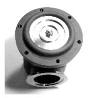
**4.** If your wastegate is fitted with a pressed upper diaphragm spring support as pictured below, proceed to the next step. (Step **5.**)
