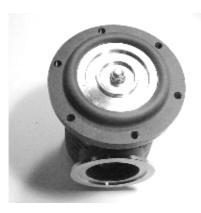
**14.** Select and fit the required wastegate spring or springs to the upper diaphragm spring support.
