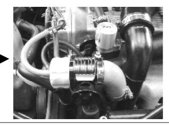
**Step 14.** Connect the short end of the 80mm Silicon bend to the Kompact boost fitting and secure with a 40mm hose clamp supplied.
