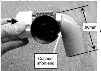
**Step 6.** Connect the pre-assembled silicon hose assembly as shown in the diagram below:
