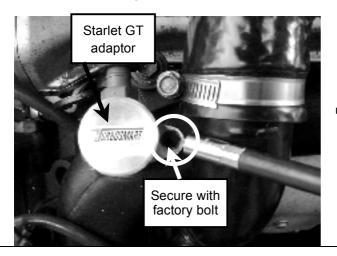
**Step 7.** Connect the 6mm ID end of the pre-assembled Silicon vacuum hose to the boost/vacuum source. Secure it with the 6mm spring clamp supplied.
