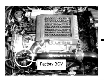
**Step 3.** Disconnect the factory vacuum/boost line from the vacuum source. Then, using a 10 mm spanner or socket, loosen the bolt securing the factory BOV.
