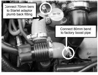
Step 18. Connect the 5mm ID end of the preassembled Silicon hose to the Kompact PB BOV.
