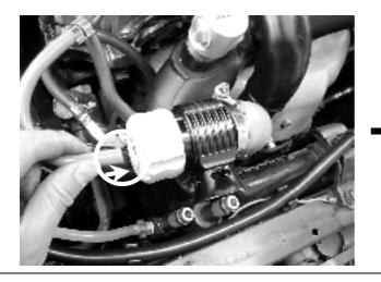
Instructions for Kompact PB installation Step 13. Install the screw-on plumb back fitting onto the Starlet adaptor. Connect the rocker cover return hose to the plastic hose fitting and secure with the factory hose clamp.
