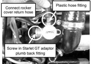
**Step 15.** Connect the long end of the 70mm Silicon bend to the Kompact plumb back fitting and secure with a 40mm hose clamp supplied.
