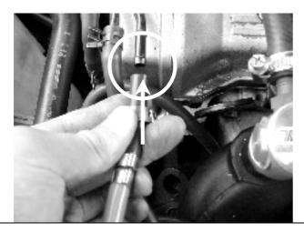
**Step 9.** Connect the short end of the 80mm Silicon bend to the Kompact SS BOV and secure with a 40mm hose clamp supplied.
