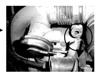
**Step 7.** Remove the bolt on the underside of the factory BOV with a 10mm socket.
