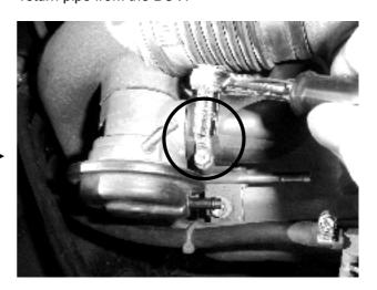
**Step 5.** Undo the hose clamp on the other end of the return hose using an 8mm socket.
