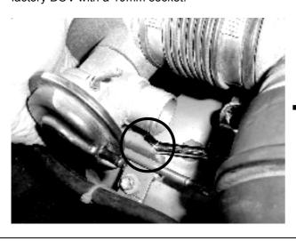
**Step 8.** Remove the bolt securing the factory BOV to the pipe flange with a 12mm socket.
