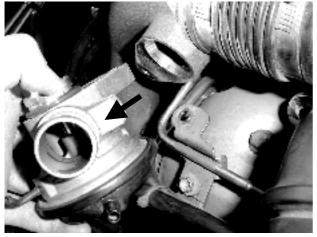
Step 11. Block off the factory return hose with the 29mm blanking plug supplied. Use the supplied 40mm
