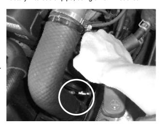
Step 17. Remove the factory intercooler pipe.
