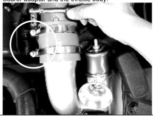
**Step 20.** Using two of the 70mm hose clamps supplied, secure the Silicon hose coupler onto the Soarer Adaptor and the intercooler pipe.
