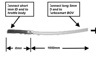
**Step 14.** Install the 6mm end of the Silicon hose assembly supplied onto the metal tube and secure with the 6mm spring clamp supplied.
