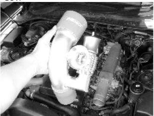
**Step 19.** Fit the adaptor between the intercooler and the throttle body. Using two of the 90mm hose clamps supplied, secure the Silicon hose coupler onto the Soarer adaptor and the throttle body.
