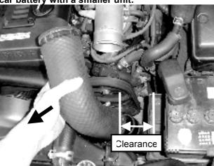
**Step 18.** Fit the Silicon hose couplers over the Soarer Adaptor. Note that the hose couplers are of different diameters to suit the larger and smaller ends of the adaptor. Install your Turbosmart BOV onto the adaptor by following the instructions included with the BOV.
