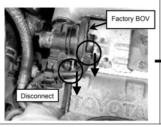
**Step 2.** Disconnect the factory plumb back hose from the factory BOV.
