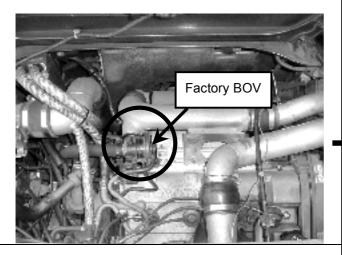
**Step 3.** Disconnect the two vacuum/boost lines from the factory BOV.
