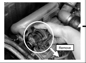
**Step 7.** Remove the O-ring on the flange of the factory BOV and install it to the flange of the MR2 adaptor. **If you are installing either a Dual Port or Plumb Back BOV, go to Step 12.**
