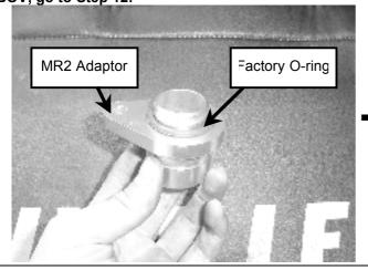
**Step 9.** Install your Turbosmart BOV onto the MR2 Adaptor by following the instructions included with the BOV.
