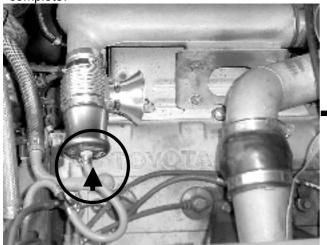
Step 13. Install the BOV and MR2 adaptor assembly, secure the adaptor with the factory bolt using a 12mm socket or wrench.
