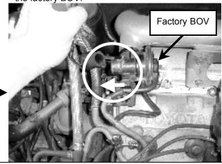
**Step 4.** Using a 12mm socket or spanner, loosen the factory bolt securing the factory BOV to the pipe flange.
