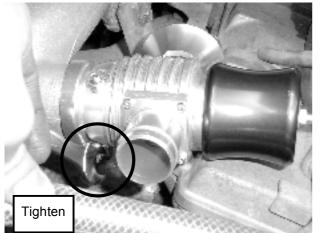
Step 15. Connect the factory vacuum/boost hose to the Turbosmart BOV fitting. Secure the fitting with the 5mm spring clamp supplied. Your installation is complete.
