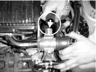
Step 11. Connect the 5mm end of the pre-assembled Silicon hose to the BOV. Secure the fitting with the 5mm spring clamp supplied. Your installation is complete.
