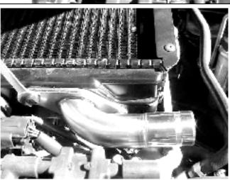
Step 6. Install your Turbosmart BOV onto the adaptor by following the instructions included with the BOV.
