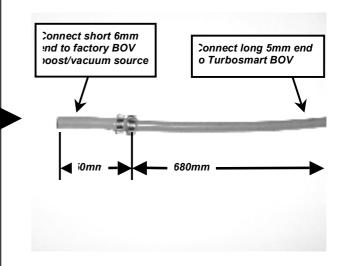
Step 9. Remove the factory vacuum/boost line from the vacuum source as shown in the diagram below:
