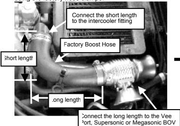
**Step 14.** Secure the adjacent hose to the BOV using the 250mm long cable tie supplied. This will prevent the BOV from moving.
