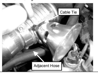
Step 11. Install your Turbosmart BOV onto the MY98 Adaptor by following the instructions included with the BOV. Go to Step 15 if you are installing a Plumb back or Dual Port BOV.
