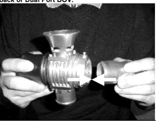
**Step 13.** Connect the 5mm end of the Silicon hose assembly onto the BOV and secure it with the 5mm spring clamp supplied.
