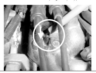
**Step 12.** When installing either a Vee port, Supersonic or Megasonic BOV, connect the short length of the factory boost hose to the intercooler fitting and the long length to the MY98 adaptor. Secure the boost hose using the factory hose clamps.
