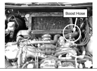
**Step 3.** Loosen the bottom hose clamp securing the boost hose to the factory BOV.
