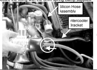
Step 17. Connect the long length of the factory boost hose to the intercooler fitting and the short length to the MY98 adaptor.
