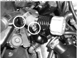
Step 12. Connect the pre-assembled silicon hose assembly as shown in the diagram below:
