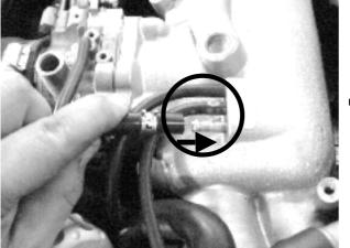
Step 14. Connect the 5mm end of the pre-assembled Silicon vacuum hose to the Kompact Supersonic 20mm BOV.
