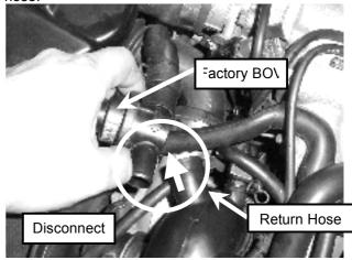
**Step 7.** Disconnect the boost hose from the boost fitting and remove the boost hose and factory BOV.
