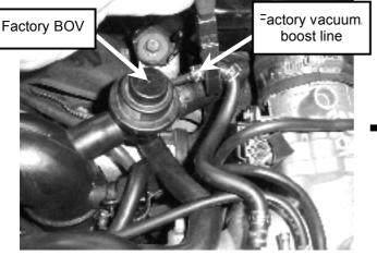
**Step 2.** Disconnect the factory vacuum/boost line from the throttle body vacuum fitting.
