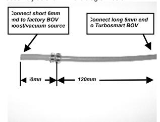
Step 13. Connect the 6mm end of the pre-assembled Silicon vacuum hose to the throttle body vacuum fitting. Secure it with the 6mm hose clamp supplied.
