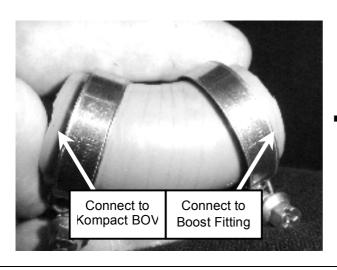
**Step 10.** Connect the 45 degree Silicon bend to the boost fitting and secure with the 32mm hose clamp supplied. Connect the Kompact Supersonic 20mm BOV to the Silicon hose.
