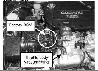
**Step 3.** Locate the factory vacuum/boost line connected to the factory BOV.
