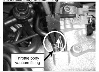
**Step 4.** Disconnect the factory vacuum/boost line from the factory BOV.
