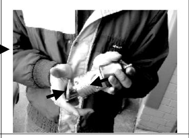
**Step 8.** Finally, insert the factory boost/vacuum line over your Turbosmart BOV nipple and secure with the 6mm hose spring clamp supplied.
