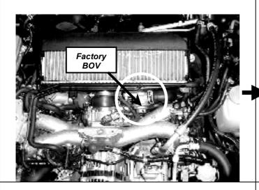
**Step 3.** Disconnect the vacuum/boost line connected to the factory BOV and undo the two nuts securing the factory BOV using a 12mm ring spanner.
