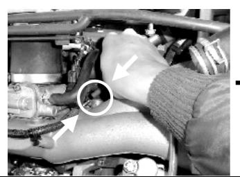
**Step 6.** Remove the whole vacuum/boost line by first disconnecting the hose from the small diameter pipe.
