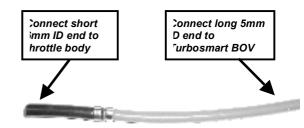
**Step 10.** Near the headlights on the left side of the engine bay, re-route the hoses feeding back to the air intake pipe. Disconnect the plastic reducer from the return hose as shown below.
