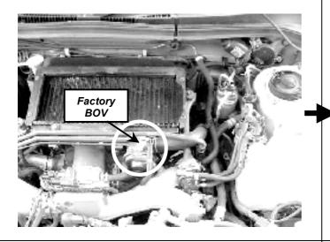
**Step 2.** Using a 12mm socket or spanner, undo the two nuts securing the factory BOV. Remove the hose clamp securing the return hose and disconnect the return hose from the factory BOV.
