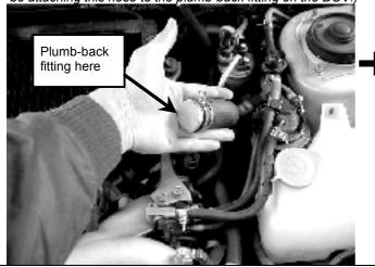
**Step 7.** Finish removing the vacuum/boost line by disconnecting it from the intake manifold to expose the fitting.
