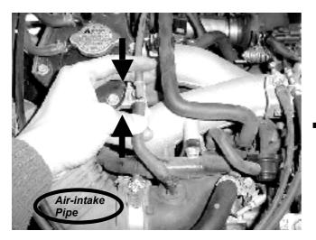
**Step 11.** Disconnect the tube connected to the small pipe. Then remove the whole tubing.
