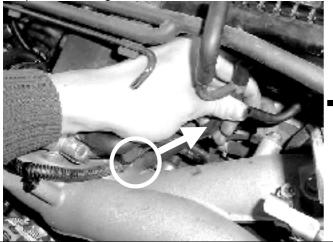
**Step 9.** Install the 6mm end of the Silicon hose assembly supplied onto the intake manifold fitting and secure with the 6mm spring clamp supplied.
