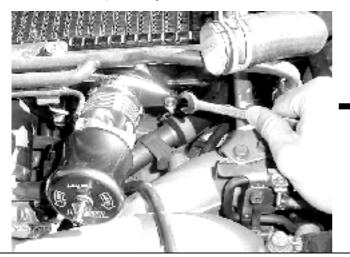
**Step 15.** Insert the 5mm end of the Silicon hose assembly over your Turbosmart BOV fitting and secure it with the 5mm hose spring clamp supplied.
