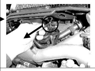
**Step 8.** Connect the pre-assembled silicon hose assembly as shown in the diagram below:
