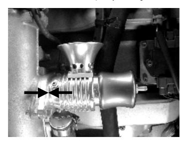
Step 12. Connect the 5mm end of the Silicon hose assembly to the Turbosmart BOV fitting. Secure the fitting with the 5mm hose spring clamp supplied.
