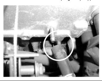
**Step 10.** Blank off the factory plumb back fitting with the supplied blanking plug. Secure the fitting with the factory hose clamp.
