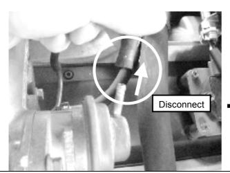
**Step 4.** Loosen the factory hose clamp securing the return hose. Remove the plumb back hose from the factory BOV and plumb back fitting.
