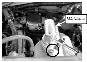
Step 8. Block off the factory return pipe with the supplied blank and the factory return hose.
