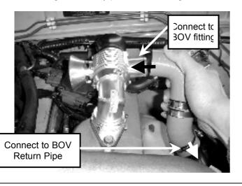
**Step 9.** Connect one end of the Silicon bend to the BOV plumb back fitting and the other end of the Silicon bend to the factory return pipe. Secure each fitting with the a 40mm hose clamp supplied.
