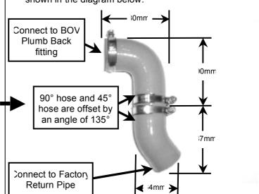
**Step 8.** Connect the preassembled Silicon bend to the BOV fitting and factory plumb back fitting:
