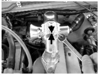
**Step 8.** Install the preassembled Silicon bend as shown in the diagram below:
