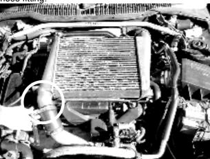
**Step 2.** Undo and remove the 2 bolts on the right hand side of the intercooler cover with a 10mm spanner or socket. Then remove the intercooler cover.
