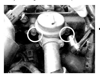
**Step 12.** Release the factory hose spring clamp with a set of long nose pliers and remove the return hose from the factory BOV.
