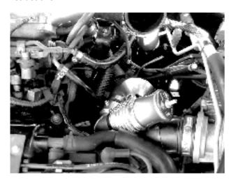
**Step 18.** If you are fitting either a Turbosmart Type III Plumb Back or Dual Port, fit the return hose onto the BOV plumb-back fitting. Secure the fitting with the factory hose spring clamp.
