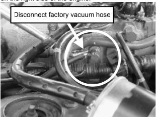
**Step 14.** Connect the 6mm ID end of 700mm long hose to the factory vacuum source and secure with 6mm spring clamp provided.
