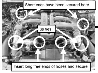
**Step 18B.** Left side vacuum/boost hose connection detail.
