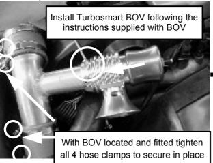
**Step 11.** Connect the two pre-assembled silicon hose assemblies as shown in the diagram below by following steps 12-17. The long 900mm version fits on the left side of the engine and the 700mm version on the right.
