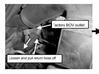
**Step 24.** Insert pill into the return hose as far as possible but at least 15mm down inside the silicon return hose as outlined below.
