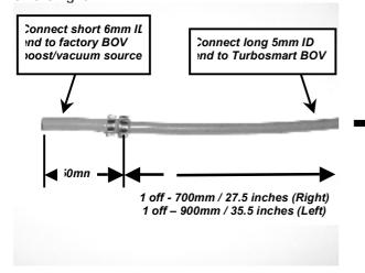
**Step 10.** Install your Turbosmart BOV onto the right side pipe by following the instructions included with the BOV. With the BOV located with adequate clearance between engine parts, tighten all four hose clamps to secure in place.
