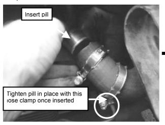
Step 25. Re-attach return hose to factory BOV and tighten. Repeat the pill insertion steps 24,24A & 25 on left side factory BOV return hose.
