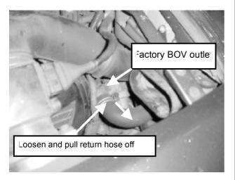
**Step 23.** With both hoses off fit supplied hose clamp over free ends loosely. This will be used to secure the pill.
