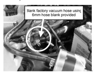
**Step 17.** Connect the 6mm ID end of 900mm long supplied hose to the factory vacuum source and secure with the other 6mm spring clamp provided. Use the other 6mm hose blank provided to blank off the factory vacuum hose
