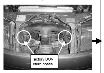
**Step 22.** Loosen and pull off left side return hose from the BOV end as shown.
