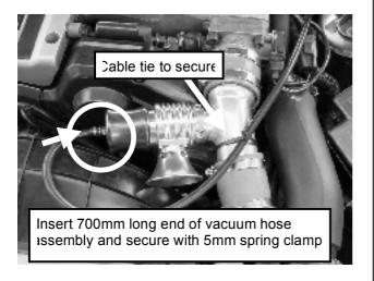
**Step 16.** Locate and remove the factory vacuum hose on the left side of the engine.
