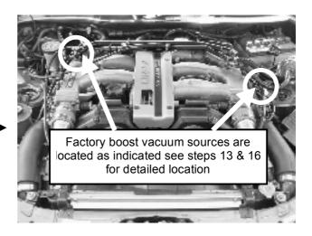
**Step 13.** Locate and remove the factory vacuum hose on the right side of the engine.
