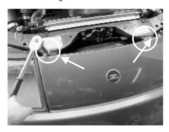
**Step 21.** Loosen and pull right return hose from the BOV end as shown.
