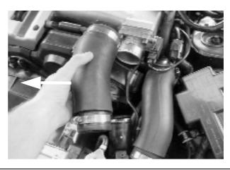
**Step 6.** Pre-assemble the left aluminium pipe, the 2" Silicon coupler and the 2.25" Silicon coupler as shown using the hose clamps supplied. Do not fully tighten clamps to allow some adjustment during installation.
