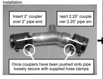
**Step 7.** Insert pre-assembled pipe kits to replace the factory boost pipes just removed. Use the short pipe on the right side as shown.
