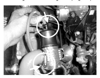
Step 18. With an 8mm socket or screwdriver, tighten the factory hose clamp at the bottom end of the factory plumb back hose. Your installation is complete.
