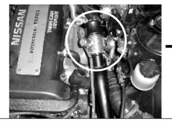
**Step 14.** Using an 8mm socket, loosen the factory hose clamp at the bottom end of the factory plumb back hose. The factory plumb back hose has to be rotated anti clockwise towards the BOV plumb back fitting.
