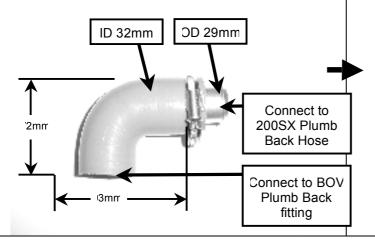
**Step 16.** Insert the 29mm OD pipe joiner into the factory plumb back hose. Secure the fitting with a 40mm constant tension hose clamp supplied.
