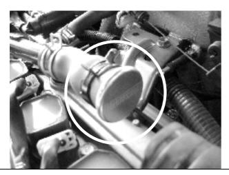
**Step 10.** Connect 3mm end of the pre-assembled Silicon vacuum hose to the throttle body fitting. Secure it with the 3mm hose clamp supplied.
