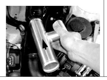
**Step 4.** Use the 70mm constant tension hose clamps supplied to secure the factory hoses to the SR20 Adaptor pipe. Tighten the hose clamps with a 7mm socket or screwdriver.
