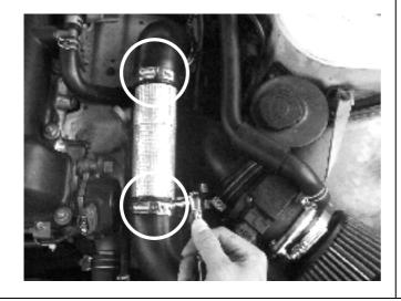
Step 2. Remove the factory pipe.
