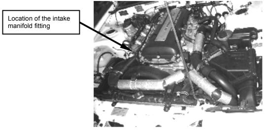
Step 6. Connect the Pre-assembled tee-piece and silicon hose assembly as shown in the diagram below:
