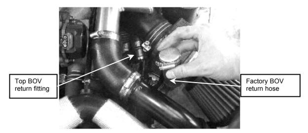
Step 10. Cut another small length of the factory BOV return hose and fit the other supplied blanking plug. Now fit this over the lower hose fitting located next to the intercooler pipe. Secure the blanking assembly with the supplied 32mm hose clamps, tighten with a 7mm socket or screwdriver.
