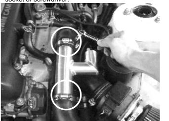
**Step 5.** Locate the intake manifold fitting connected to the factory boost/vacuum line. It is on the left hand side of the engine bay. Remove the factory boost/vacuum line to show the intake manifold fitting.
