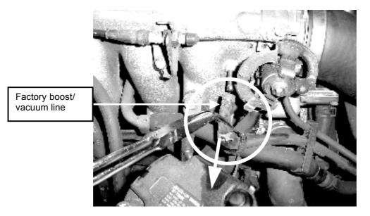
**Step 10.** Connect the pre-assembled tee-piece and silicon hose assembly illustrated below, to the exposed fitting on the intake manifold.
