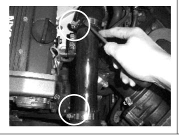
**Step 2.** Undo the bolts that secure the factory pipe, using a 12mm socket.
