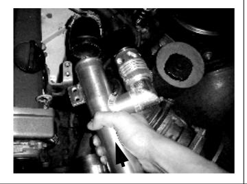
**Step 7.** Secure the CA18 Adaptor onto the mounting by tightening the two factory bolts with a 12mm socket.
