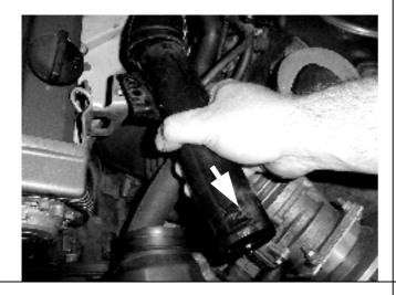
**Step 5.** With the BOV fitted, insert your CA18 Adaptor between the turbo outlet and the intercooler pipe.
