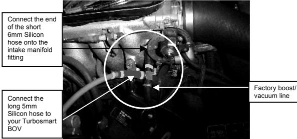
Step 12. Connect the 5mm Silicon hose to the BOV and secure it with the 5mm spring clamp supplied.
