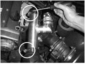
**Step 8.** Locate the intake manifold fitting connected to the factory boost/vacuum line. It is on the left hand side of the engine bay.
