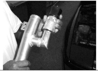
**Step 6.** Use the 70mm constant tension hose clamps supplied to secure the factory pipes to the CA18 Adaptor pipe. Tighten the hose clamps with a 7mm socket or screwdriver.
