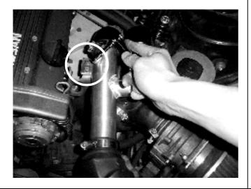
**Step 4.** Install your Turbosmart BOV onto the CA18 Adaptor by following the instructions included with the BOV.
