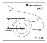
**3.** After installing the tires, measure the distance from the wheel center and the fender edge as shown in the Figure, and confirm that it corresponds to the reference value shown below.
