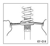
2. After adjusting to the appropriate height, use the adjustment wrench included with the Product to lock the lower spring seat.
