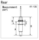
1. After installing the shock absorber on the vehicle, measure the area marked in the Figure, and adjust to match the reference values shown.
