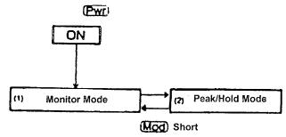
\*Note: The EVC does not have to be in peak/hold mode in order to record the peak boost level.
