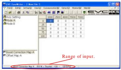
Correction will be performed according to the boost correction value of the throttle position, RPM, and speed in addition to the set boost in Mode A/B.
