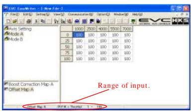
This offset is used to make fine adjustments to the set boost in Mode A/B relative to throttle position, RPM, or speed.
