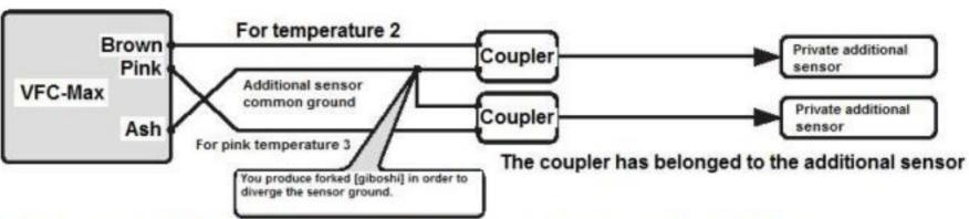
It diverges the ash of VFC into 2 crotches. For temperature 2 in sensor, brown ash. For temperature 3, to connect the coupler to the pink ash respectively in the sensor, please connect with the sensor itself.
