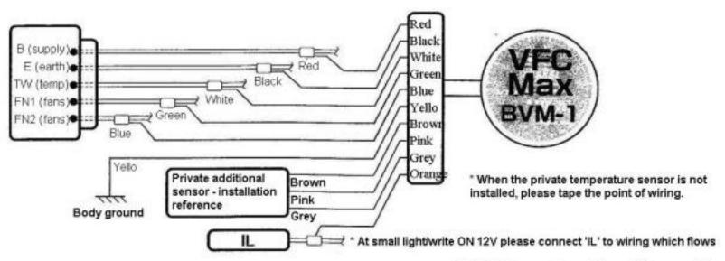
OPTION: The optional adapter for the electromotive fan highest fast rotary circuit of FD3S (the VA-2 ¥3,675 itself price ¥3,500) there is setting. " This adapter does not turn on the switch of the air conditioner and also the [te] the electromotive fan is the part which it tries to be able to turn at full speed. As for the electromotive fan independence control of medium speed high speed becomes possible, by installing this adapter, but low-speed operation becomes impossible
