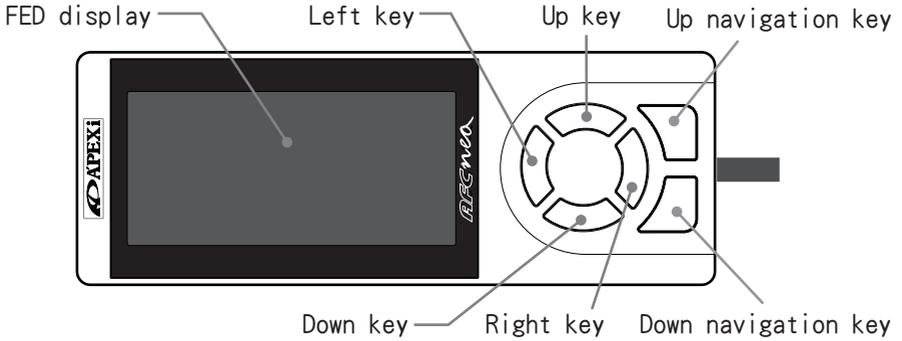
When the left/right-side installation function is set to "Left," the names are assigned as follows.
