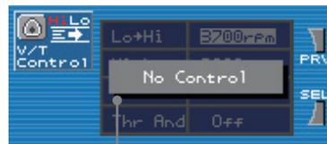
It is displayed as "No Control" and "V/T Control" stops functioning.
