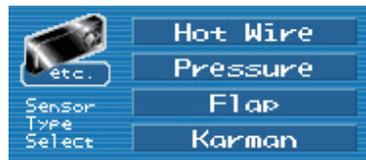
For “Hot Wire,” “Pressure,” and “Flap” , press the Right or lower navigation key to go to the sensor number selection window.
