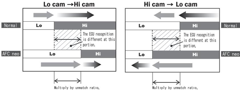
When VTEC changeover point has been changed in the V-AFC II, improper fuel injection is performed because the ECU does not recognize the actual cam status. This correction is performed so that the fuel adjustment may not be shifted at that time.
