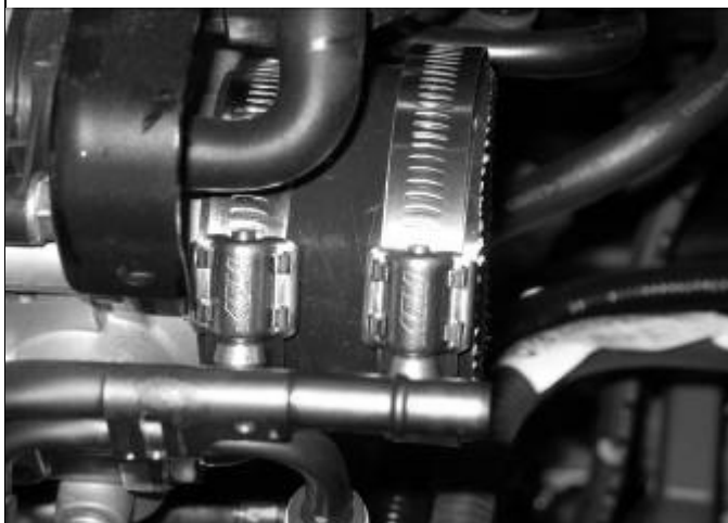
e) Install the supplied reducing coupler onto the throttle body using a #40 and #44 hose clamp as shown.
