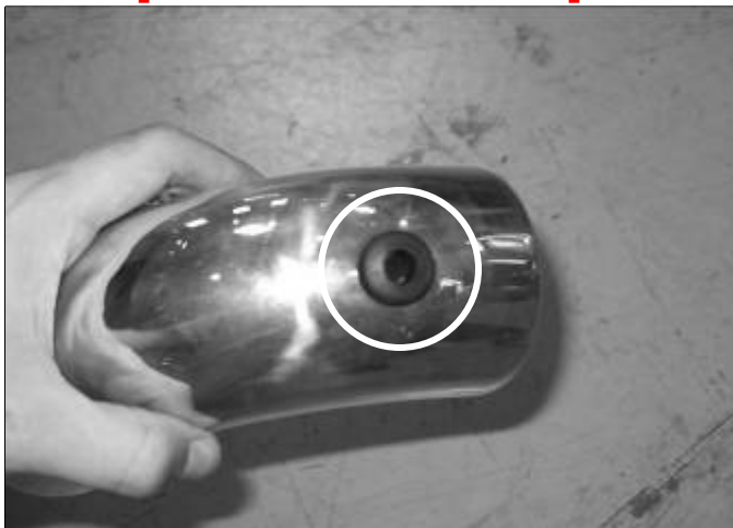
c) Install the rubber grommet into the hole on the short upper pipe as shown.
