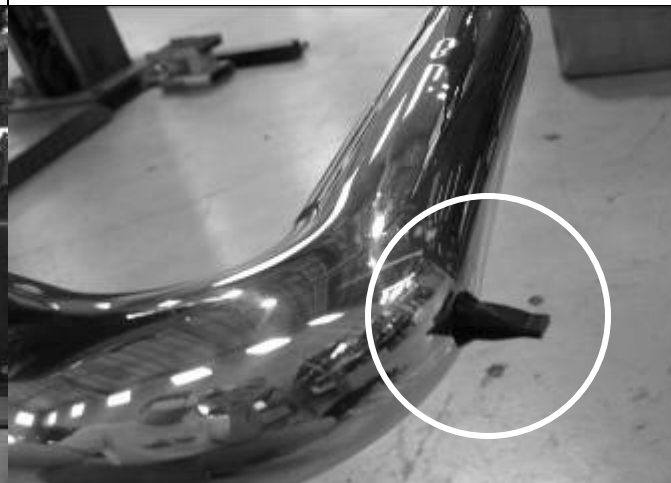
h) Locate the hole on the lower inlet pipe and insert the supplied duck bill drain as shown.
