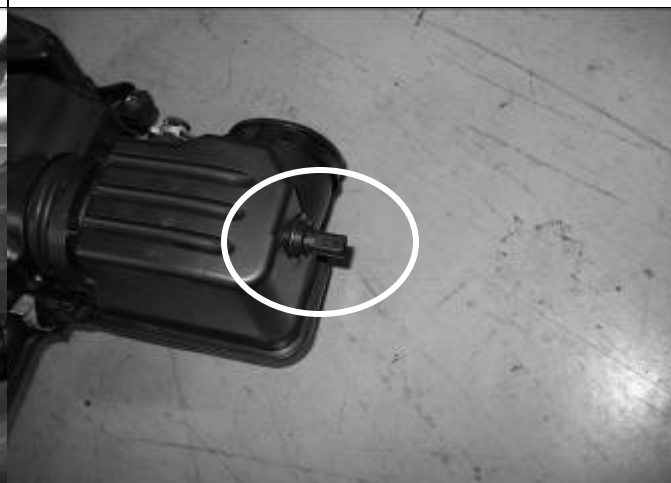
p) Carefully remove the IAT sensor from the previously removed resonator and air filter housing.
