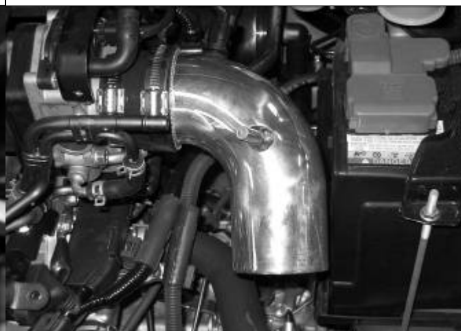
f) Slide the short upper inlet into the throttle body with the IAT sensor facing the firewall. If clearance is needed, loosen the battery mount and slide battery away from pipe.
