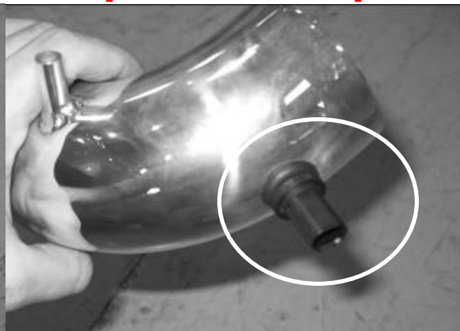
d) Carefully install the IAT sensor into the grommet. Fitment may be tight, if so use soapy water to ease installation..
