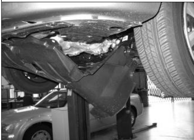
m) Unclip the underbody tray from the driver's side fender liner and let it hang to gain access behind the front bumper as shown.
