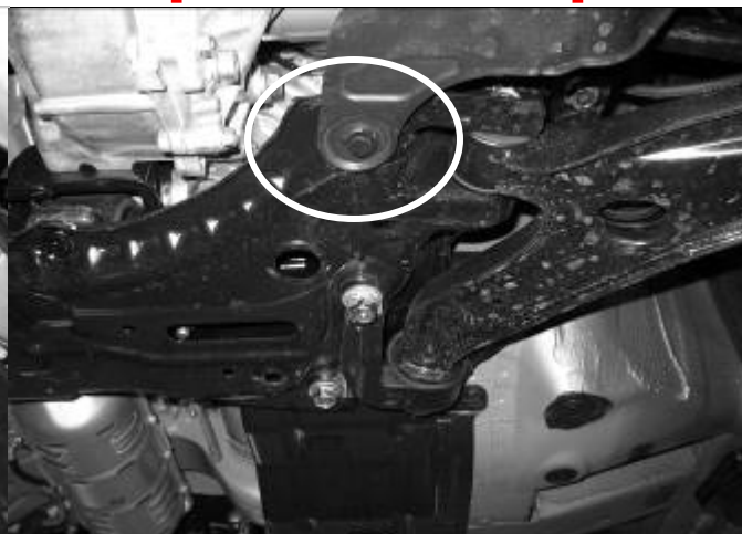
l) From underneath the vehicle remove the plastic retaining clip located on the driver's side subframe.
