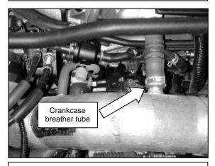
f. Install the crankcase breather tube on the intake pipe and secure it with the stock spring clamp.
