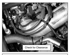
j. Check for proper hood clearance. Re-adjust pipes if necessary.
