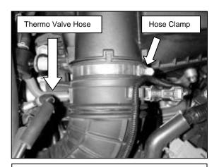
f. Remove the hose clamp securing the stock upper intake tube to the filter box. Remove the thermo valve hose. Remove the stock upper intake tube from the vehicle.
