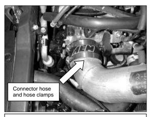
d. Install the supplied connector hose onto the throttle body and the intake pipe. Install the two supplied hose clamps on the connector hose.
