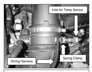
e. Remove the wiring harness from the rubber holds in the stock upper intake tube. Disconnect the inlet air temp sensor wiring harness. Loosen the spring clamp securing the inlet air temp sensor and remove. Set the inlet air temp sensor aside as it will be reinstalled on the AEM® intake system.
