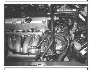
I. Factory air box system removed from the vehicle.
