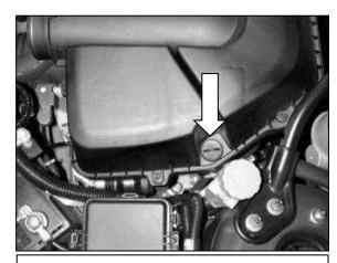
h. Remove the rubber plug from the filter box.
