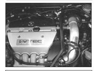
i. AEM® intake system installed
