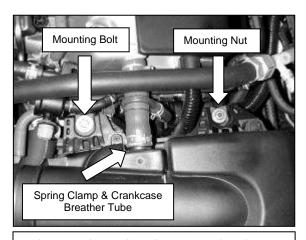
g. Loosen the spring clamp securing the crankcase breather tube and remove from the filter box. Remove the mounting bolt securing the filter box. Remove the mounting nut securing the filter box.
