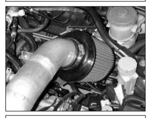
h. Install the AEM<sup>®</sup> air filter onto the end of the intake pipe. Install the supplied hose clamp to secure the filter on to the intake pipe.
