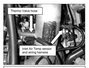
e. Install the thermo valve hose on the intake pipe. Plug in the inlet air temp sensor wiring harness.
