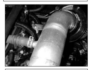
g. Install the intake pipe over the aluminum spacer. Use the supplied nyloc nut and washer to secure the intake pipe.
