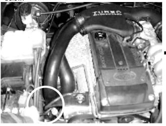
**Step 3.** Flip over the factory manifold to reveal the factory BOV. Undo the two hose clamps that are fastening the factory BOV to the boost and exhaust hoses and remove the factory BOV.
