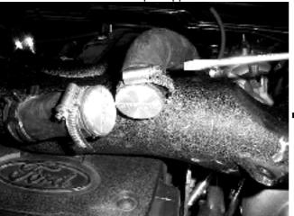
**Step 6.** Remove the black rubber pipe connecting the intercooler to the factory manifold by removing the spring hose clamp located within the circle pictured below.
