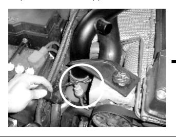
Step 12. Connect the 5mm ID Silicon hose supplied onto the factory tee-piece. Secure the fitting using a 5mm spring clamp supplied.
