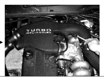
**Step 7.** Connect the Silicon bend hose coupler to the bottom end of the XR6 adaptor. Trial fit the adaptor. Leave about a 20mm gap between the end of the adaptor and the end of the factory pipes to allow for engine movement.
