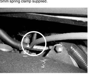
Step 13. Connect the Silicon hose to the top of your Turbosmart BOV. Secure the 5mm Silicon hose using the remaining 5mm spring clamp supplied
