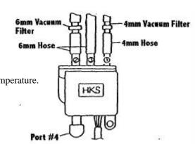
Port #1- Connect to an uninterrupted intake manifold pressure source after the throttle body such as a compressor bypass signal line using the 4mm hose.
