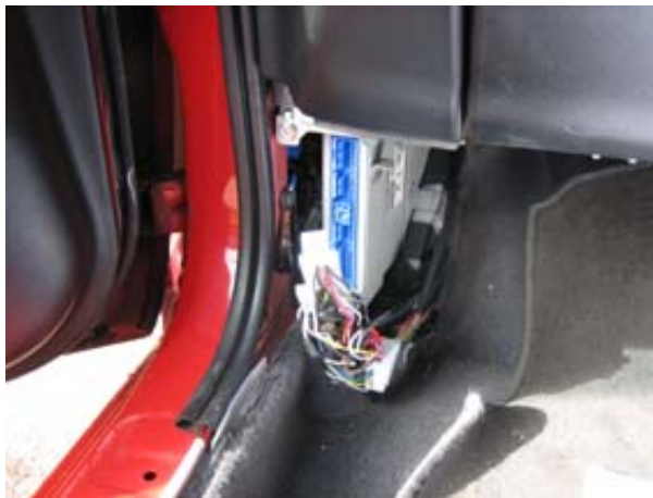
This picture shows the wires on an S14a separated from the rest by the knife
