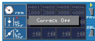
When correction is OFF, the screen is displayed as shown at left, and air correction factor  $\pm 0$  is assumed.
