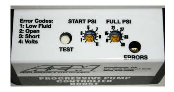
Adjust the "Start PSI" value by setting the dial to approx 25% of the vehicles maximum boost. Adjust the full-in value to your maximum boost (up to 38 PSIg of boost).
